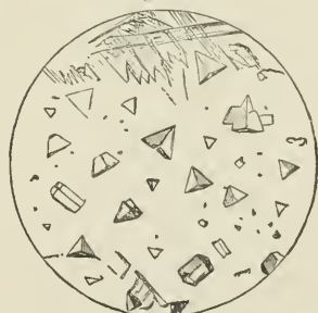
Crystals of Tartar Emetic, magnified 30 diameters.
